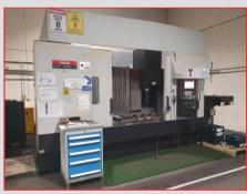
\*Mazak VTC - 200C - II CNC Vertical Travelling Column Machining Centre with CNC Control Mazatrol 640 M, 30 ATC, 12000rpm, Spindle, Table size 2000mm x 510mm, Max load on the table 1000kgs, Machine Weight 8260kg (2004)
