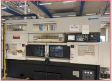
Mazak Multiplex 6300 Turning Centre with Mazatrol 640T Control, Flex-GL200F Gantry Loading System (2004)
